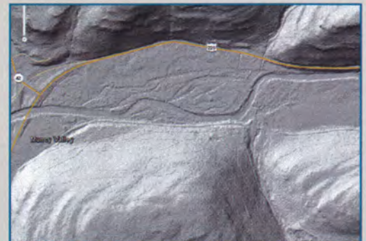
Figure 6. A LiDAR digital terrain image of Muncy Creek, showing the braided, or multi-threaded channel pattern visible on the valley floor, with the artificially straightened and deepened channel dredged to drive logs downstream.
