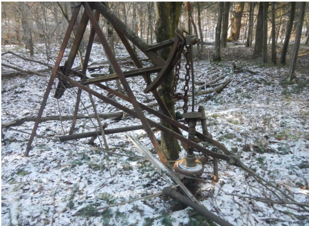
Orphan well with tree growing in the ancient pumping unit
