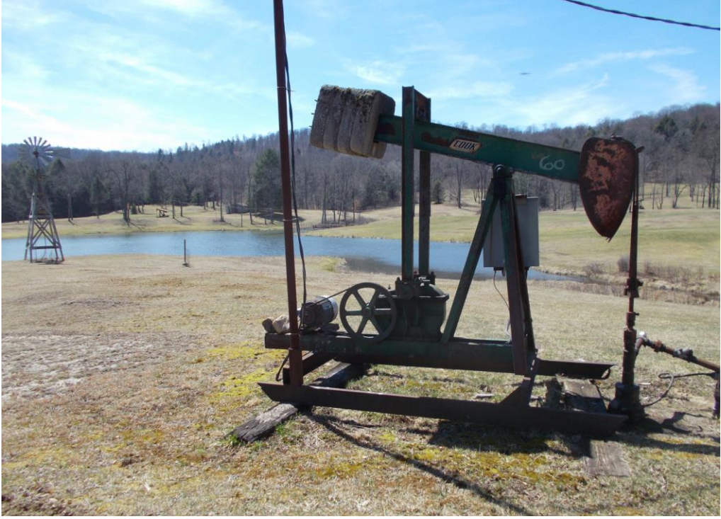
Modern pumping unit located at Cameron Energy headquarters parcel
