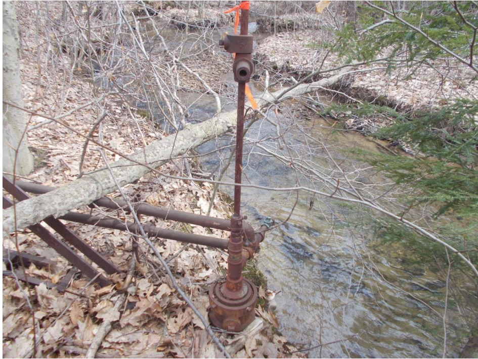
Orphan well located on stream bank (such location not allowed in modern times)
